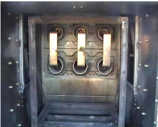
Figure 4. Test result with light and current based protection.
