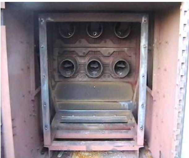
Figure 3. Test result with 500ms arcing time.
