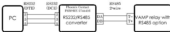
Figure 1. Test system. A PC connected with an RS232 cable to a Phoenix Contact 232/485 converter. The converter is connected with a twisted pair to a VAMP relay.
