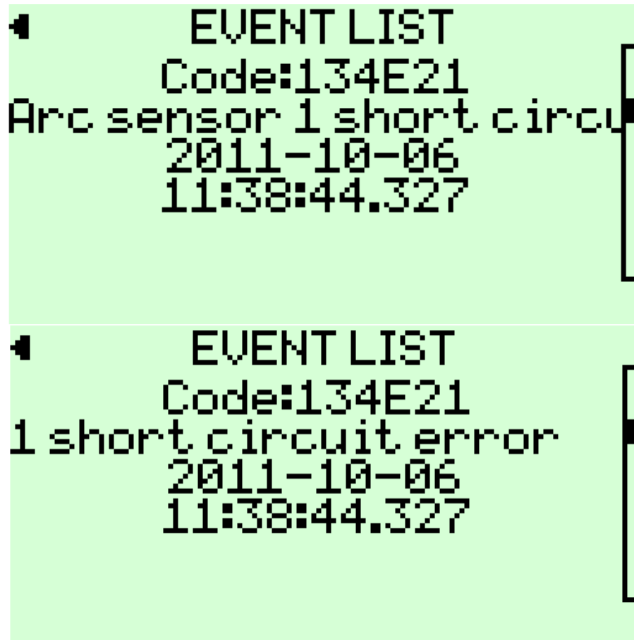
Figure 15: 'Arc sensor 1 short circuit error'
